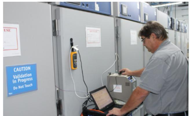
*Figure 5. IQ/OQ/PQ validation must be performed when a GMP storage facility is first commissioned, followed by appropriate requalification intervals.*
