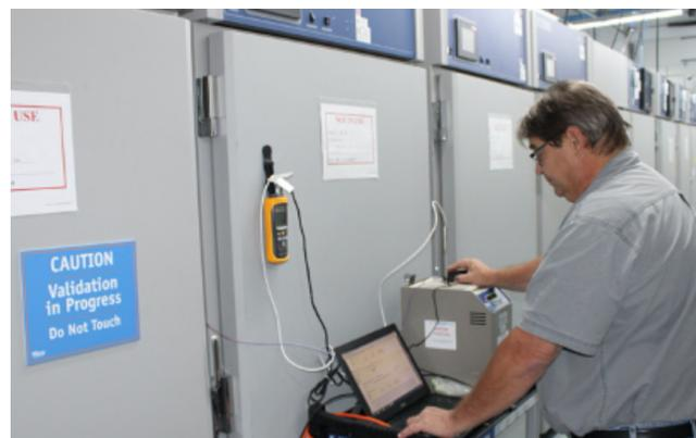
*Figure 5. IQ/OQ/PQ validation must be performed when a GMP storage facility is first commissioned, followed by appropriate requalification intervals.*
