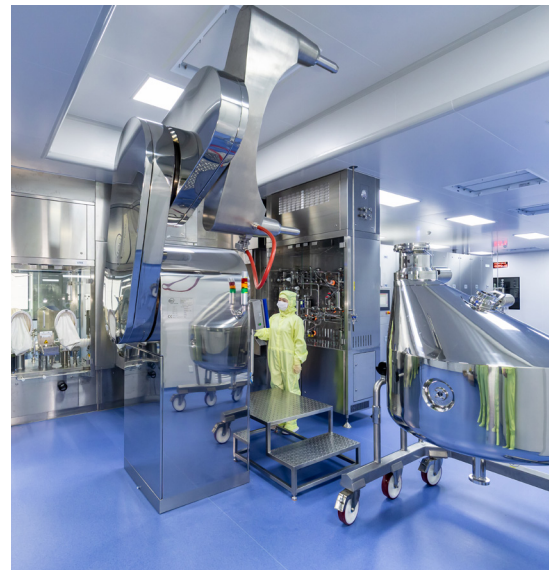
Robotic arm and processing tank within the fill-finish cleanroom at Altruist Biologics, enabling automated material transfer to an isolator ( HTTPS://WWW.ALTRUISTBIO.COM )
